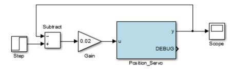
Change the "Final value" parameter of the step to 0.5 and the "Gain" parameter in the gain block to 0.02. Set the simulation stop time to 2 seconds.
