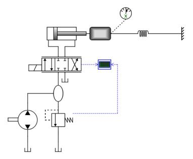
To communicate between Simulink and Hopsan we need some interface ports. These are defined by *Interface* components in Hopsan. We want to use control signal to the valve for input, and the actual position of the piston for output. Add one input and one output component:
