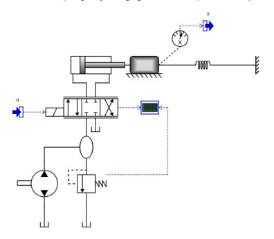
Also change the damping parameter  $(B_p)$  in the piston component to 1000. Then click *save as* (not *save*!) and overwrite the model *in the exported directory*. This is the model used by Simulink. Then simulate from Simulink again and look at the results. The results are now different, even though we did not re-export the model.
